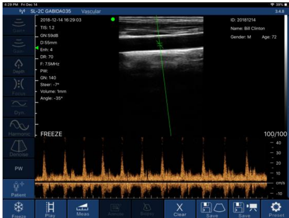
Image 3-4 Pulse Doppler Imaging Mode
